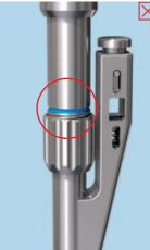
**3. Mount torque limiter and deploy screwdriver insert** Mount the torque limiter on the screwdriver handle.
