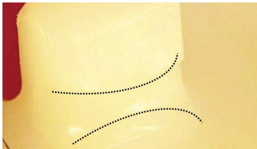
Figure 2. Photograph of a retrieved PS polyethylene insert demonstrating anterior spine impingement and subsequent wear.
