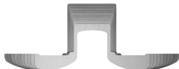
Figure 7: Diagram of the coronal cross-sectional geometry of the ATTUNE Knee femoral component demonstrating how the intercondylar box width, and subsequent intercondylar bone resection required, lessens with decreasing femoral component size.
