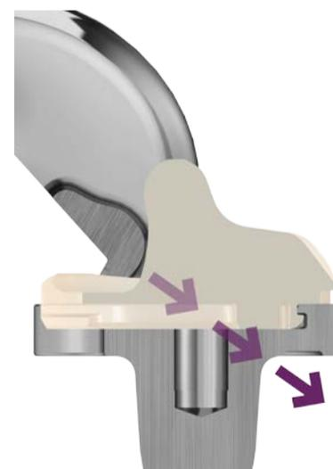
Figure 4B: Cross-sectional diagram of the SOFCAM at 145° of flexion demonstrating contact at the base of the spine where polyethylene strength is maximized.
