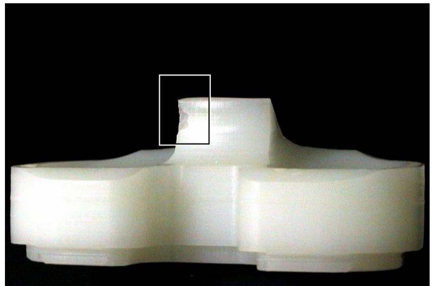
Figure 1. Photograph of a retrieved PS polyethylene insert demonstrating eccentric medial spine wear.
