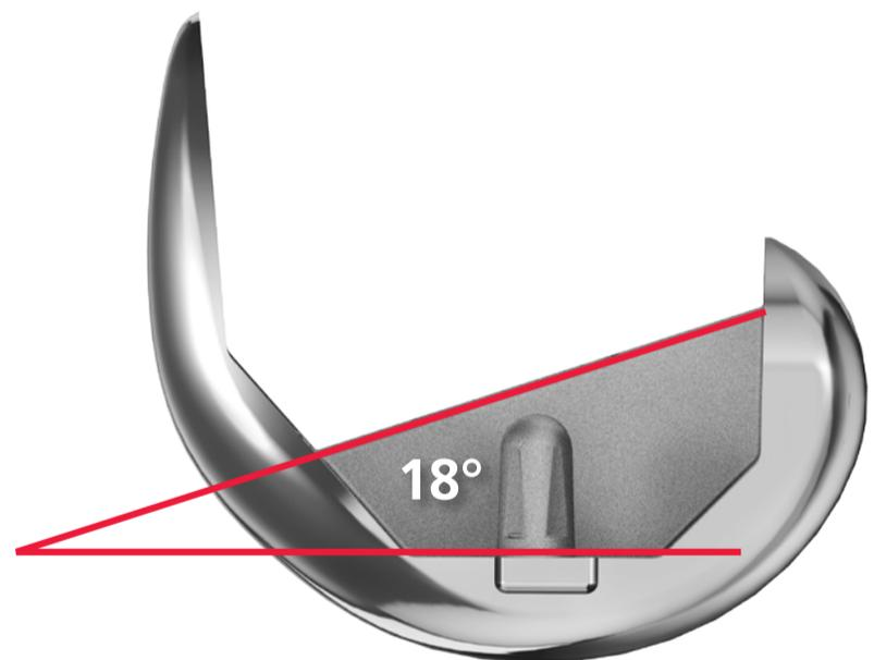
Figure 6: Sagittal view of the ATTUNE System femoral component demonstrating the angular (18°) intercondylar box which gives rise to less intercondylar bone removal.
