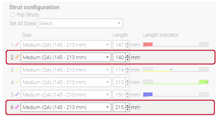
Figure 91 – Frame Configuration – Missing Strut length indicators.
