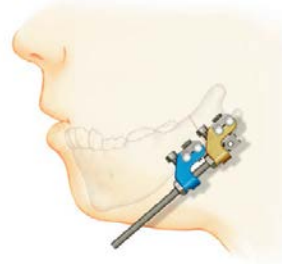
Single Vector Distraction (distraction up to 70mm)
