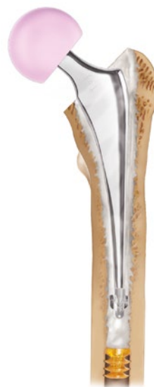
Figure 8: Representative example of a hip implant with bone cement fixation.
