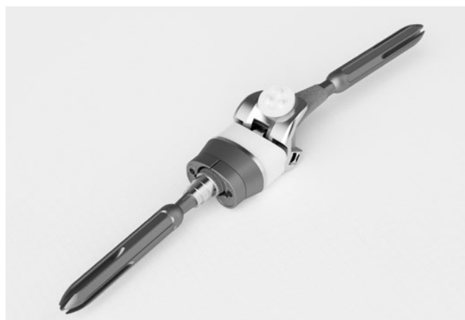
Figure 3: Worst-case total knee construct (codes in Appendix 1) used for FTIA testing. 19
