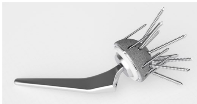
Figure 4: Worst-case hip construct (codes in Appendix 3) used for FTIA testing. 20
